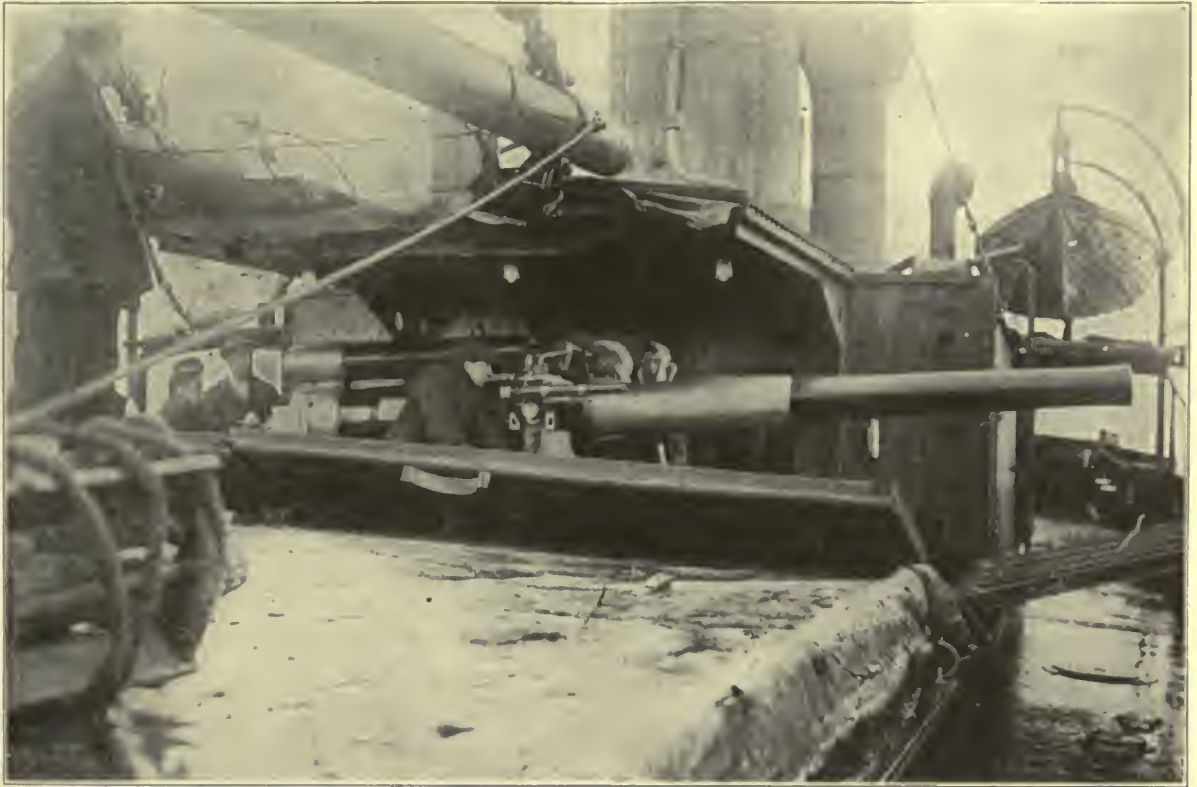
Hidden mysteries of the famous "Q" ship of the British Navy, H. M. S. Suffolk Coast, used as a decoy to capture or destroy submarines. View of the dummy deckhouse, showing the gun which was concealed until the iron doors fell at a signal from the bridge
